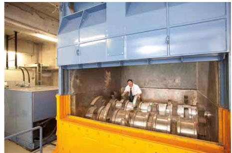
Figure 1b: Hook shredder SID XLC 7300 with open ejection door for unshreddables
