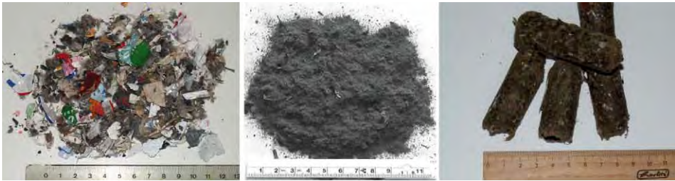
Figure 4: Examples of different qualities of solid recovered fuels used in coal-fired power plants (left: pelletized SRF < 10\text{ mm} ; middle: SRF fraction from the mechanical-biological treatment plant Kahlenberg/Maximum Yield Technology process; right: SRF hard pellets)
