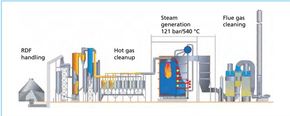
Figure 3: Conceptual diagram of a waste gasification power plant
